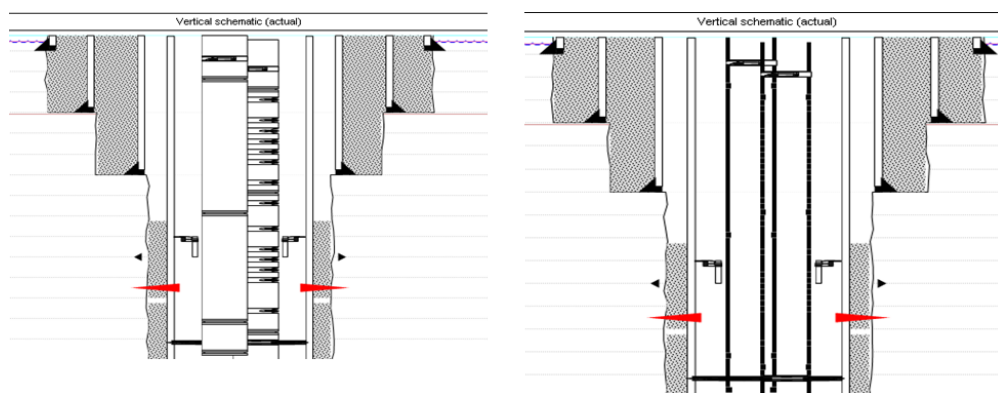
The schematic on the right side has alternate barrier icons substituted for tubing components defined as Mandrels, Tubing, Nipples, etc. SSSV and packers are drawn with the normal icons.
